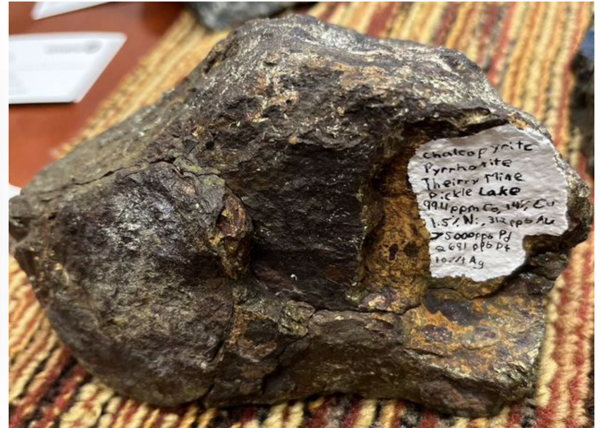
High-grade sample from Thierry Mine showing 14% Cu, 1.5% Ni, 994ppm Co
